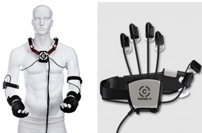
Figure 2.8: ControlVR system and a closeup of one of the gloves featuring inertial sensors.
