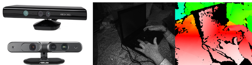
Figure 2.2: From right to left: Kinect and Xtion devices. Projected IR dot pattern. Depth map constructed from the dot pattern. Source: http://asus.com and http://en.wikipedia.org/
