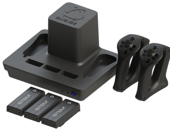
Figure 2.6: STEM controllers, external base station and three sensor modules. Source: http://store.sixense.com/
