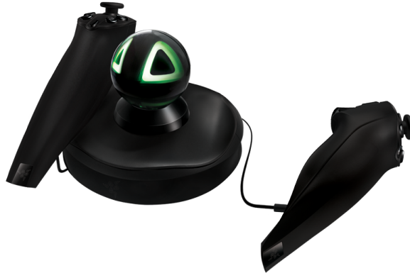
Figure 2.5: Razer Hydra controllers and external base station.
