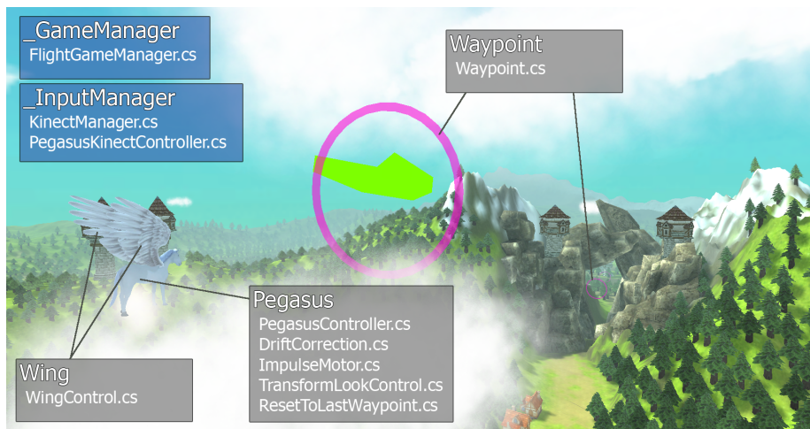
Figure 3.13: Pegasus Flight scene showing the relevant GameObjects and attached scripts.
